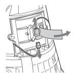
6 Remove the 2 screws, then remove the battery cover and the battery pack.
